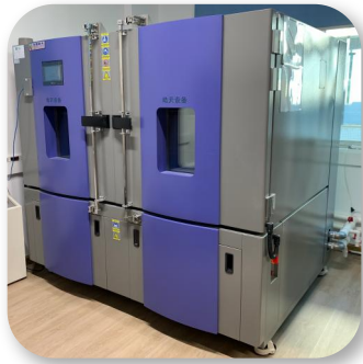
Constant Temperature and Humidity Test Chamber
